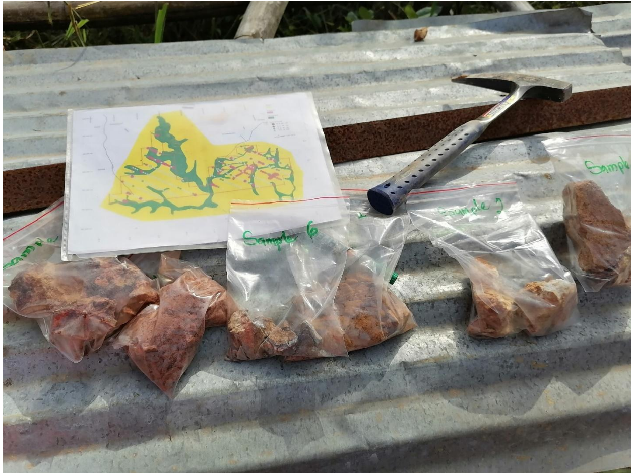
Figure 3. Collected samples that have been described, bagged and labeled during the field work. All samples collected during this visit were analyzed for gold.
