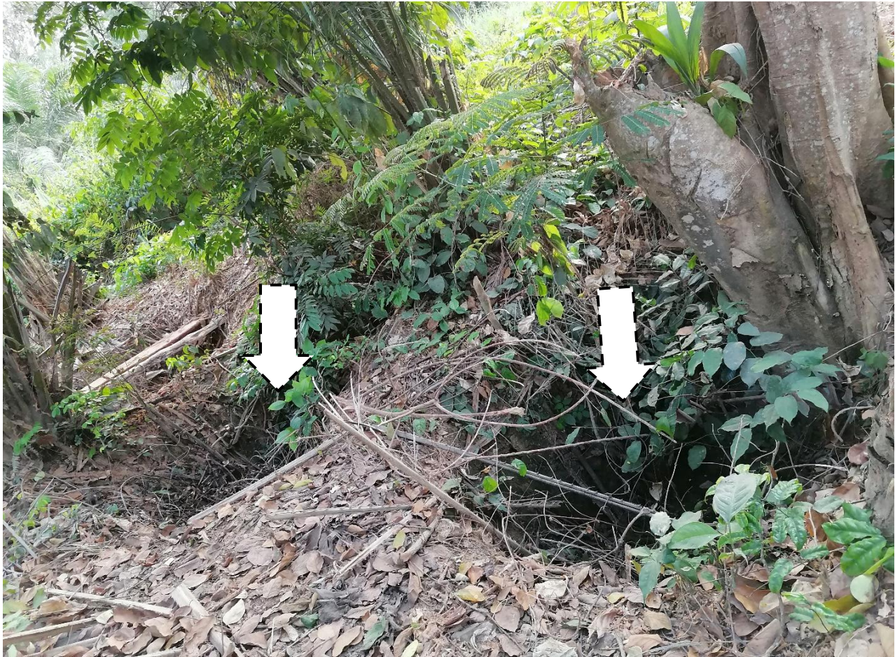
Figure 7 . At Nyinahin. Dug-out pits by artisanal miners, who previously mined quartz-veined rocks in this area. Geochemical analysis of samples collected from some of these pits during the current field visit yielded appreciable gold concentrations and indicate a great potential for gold mineralization in deeper parts of this area.
