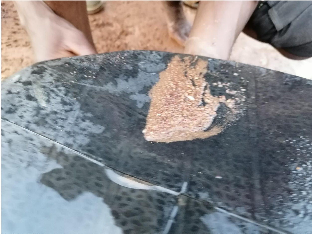
Figure 11. At Nyinahin. Panning of soils in water to separate tiny flakes of gold from soil samples. Gold flakes were seen with the naked eye by the geologist (author).
